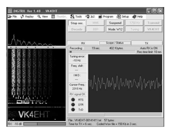
Above is an example of the DIGTRX screen as it is recording an incoming signal. The "Scope/Status" window emulates an oscilloscope. The spectrum display (top left) shows the 8 carriers and in this example shows a drop in level of the higher frequencies. The waterfall display scrolls downwards showing the ID sent at the beginning of transmission followed by the 8 carriers (about 19 seconds into the transmission as indicated in the recording panel). Below this is the audio level in bar graph form.
