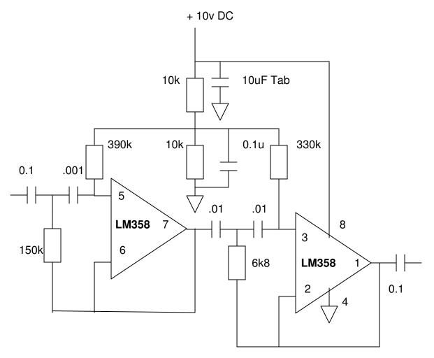
Audio Input T3 board, pin 74 Audio Output T3 board, pin 71 +10v T3 board, pin 3 Ground T3 board, pin 8
